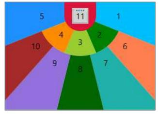
The ideal coverage shape in this case is Semi-Circular as it provides full coverage of the room while the BMA 360 is physically mounted off center. Here is another image of the classroom with this beam pattern overlaid.
