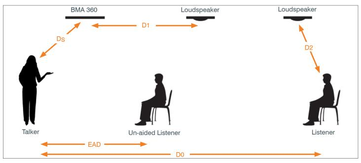
It's easy to see the purpose of Voice Lift is to Lift audio heard by listener at distance D0, to the equivalent level heard by the un-aided listener at EAD.
