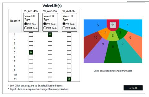
Adding Processing blocks in line with these VL Channels will even further expand your control and tuning capabilities.
